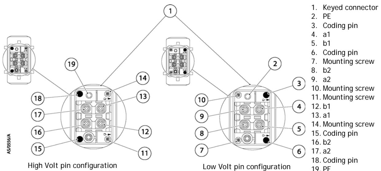
Figure 9 - Method for connecting phase wires
