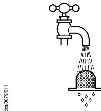
Figure 14 - Flush the filter
