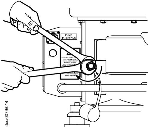
Figure 16 - Refit the filter inlet fitting
