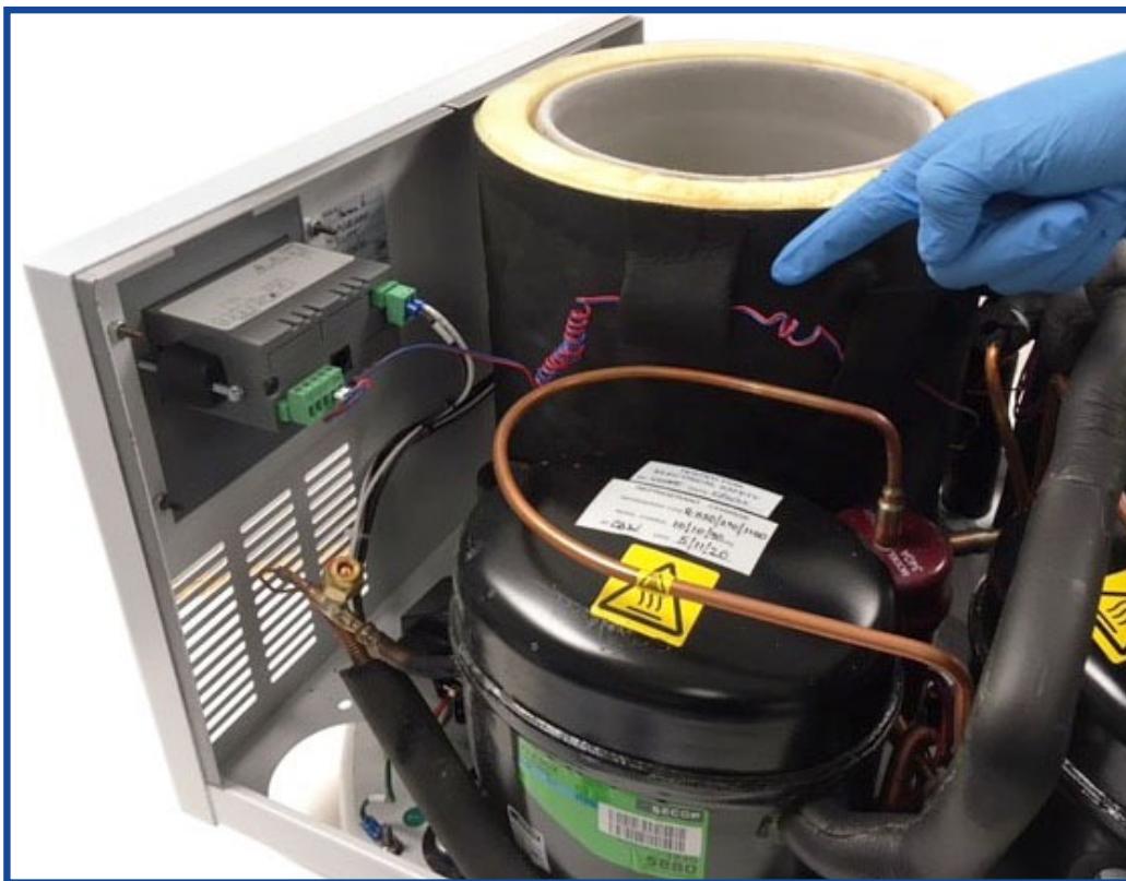
Figure 5 - Location of Type T Thermocouple
