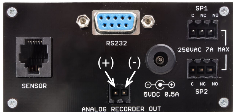
Figure 5 - XG-120 rear panel connections
