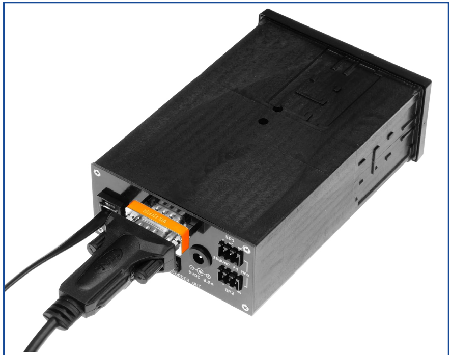
Figure 7 - Connect the null modem adapter and cable
