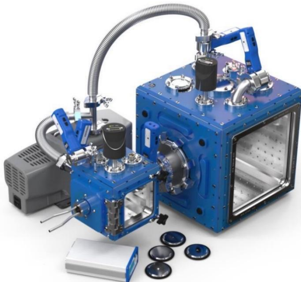
Figure 7: Off-the-shelf explosive decompression test system with test and boost chambers, electronic butterfly valves, capacitance manometers, gauge controller, and IDP-3 vacuum pump. The kit also includes assorted orifices for fine tuning the decompression speed (Ideal Vacuum Products Part Number P1010268).
