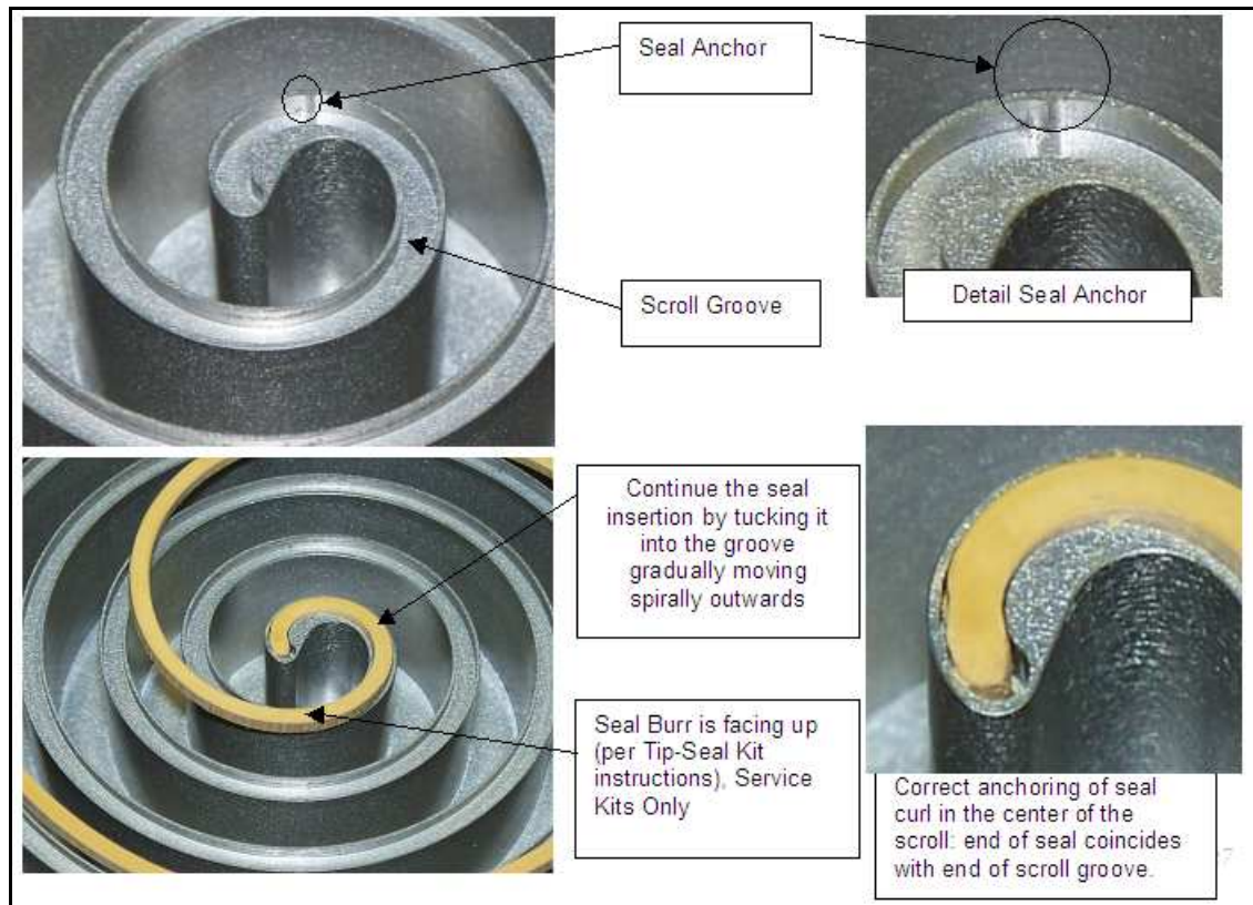
Figure 11 Tip Seal Seating
