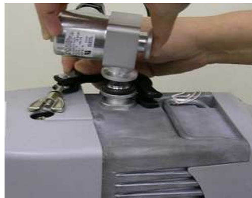
Figure 9 Mount Inlet Valve with IDP-3 Pump
