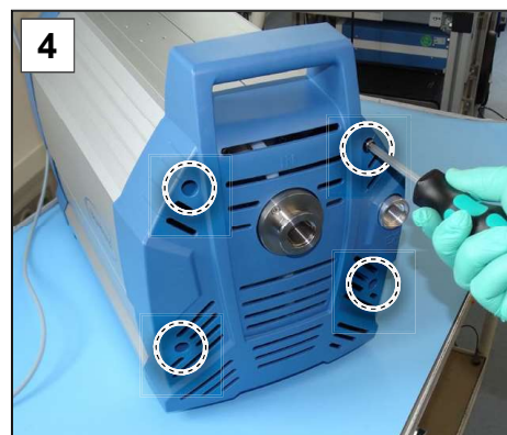
4. Wind in the 4 screws of the front housing section; hex key size 4.
