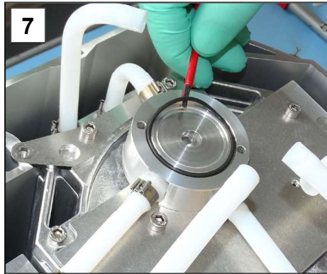
7. Carefully remove the used pressure relief valve and the O-ring, e. g., with a narrow flat-head screwdriver.
