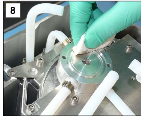
8. Clean the pressure distributor if necessary.
