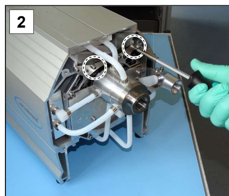
2. Wind in the 2 outer screws of the side panel retaining plate at the front; hex key size 4.
