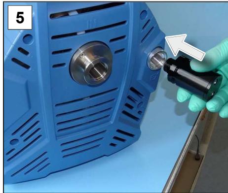
5. Screw the silencer in the thread at the outlet..
