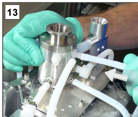
13. Push the molded hoses back into place on the hose nozzles.
