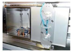
Load the material to be evaporated into the boat or crucible to be used.
