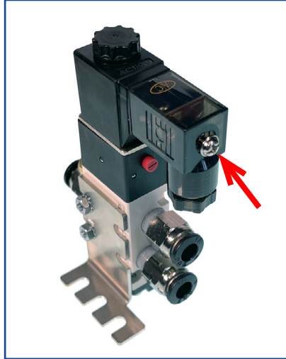
Figure 7 - Remove connector screw
