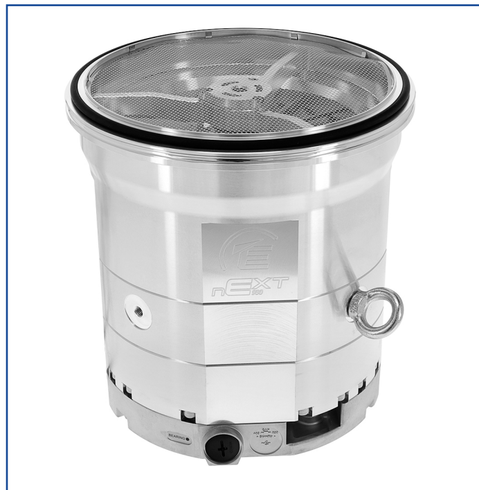
Figure 17: Edwards nEXT930D turbo pump (P1012398) fitted with an ISO-K 200 centering ring with fine inlet screen (P1012402). This is an example of a turbo pump which cannot be oriented with the inlet facing down.
