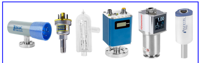
Figure 8: Left to right; IVP convection-enhanced Pirani gauge (P1010258), Teledyne-Hastings DV-6M thermocouple gauge (P102046), IVP hot cathode ion gauge (P102041), MKS Granville-Phillips® 355 hot cathode Micro-Ion® gauge (P1012041), Leybold Penningvac® PTR 90 N Pirani + cold cathode combination gauge (P109872), Inficon PSG500 Pirani gauge module (P1010832).
