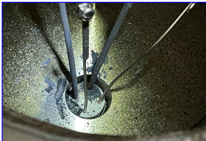
Figure 11: A combination power + thermocouple vacuum chamber feedthrough (P108066) used with a process that produced a sticky organic residue. The copper wires were carrying ~20 A of current at 208 VAC and got very hot, carbonizing the organic residue. Eventually the electricity arced to the grounded steel chamber, resulting in a blown fuse, a ruined experiment, and a lengthy cleanup (see Dirty Processes - Scum, page 14 ).
