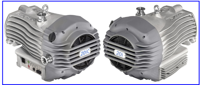
Figure 7: Left to right: An Edwards corrosive-rated nXDS20iC dry scroll pump (P105129), and a standard nXDS20i dry scroll pump (P105132). Both have identical pumping performance for non-corrosive gases. The corrosive-rated nXDS20iC can handle more corrosive chemicals because it is equipped with Chemraz® seals and stainless steel springs. A standard XDS20i can be converted into a nXDS20iC with a conversion kit (P109572).
