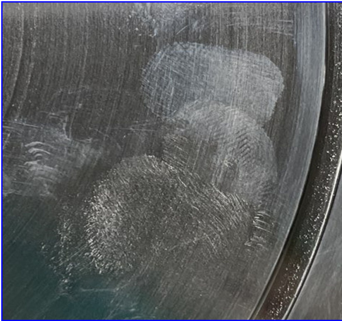
Figure 5: Oily fingerprint residue on a machined stainless steel ISO-K DN 160 blanking plate (P101684). Wear clean gloves when handling vacuum equipment. It saves time and prevents problems.
