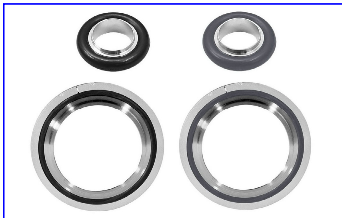
Figure 9: Standard KF and ISO Viton O-rings can be replaced with Kalrez for greater chemical and thermal stability. From left to right; top: KF-16 centering ring with Viton O-ring (P101242) and with Kalrez O-ring (P106147); bottom: ISO 100 centering ring with Viton O-ring (P101768) and with Kalrez O-ring (P108590).
