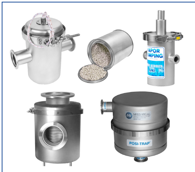
Figure 14: A sample variety of traps for protecting pumps from condensable vapors. From left to right; top: inline molecular sieve trap (P103869), zeolite pellets for hydrocarbon and oil removal (P105408), Ideal Vacuum inline liquid nitrogen cooled trap (P103849); bottom: right-angle water-cooled trap (P103874), Posi-Trap right-angle media trap with interchangeable media elements (P1011050).
