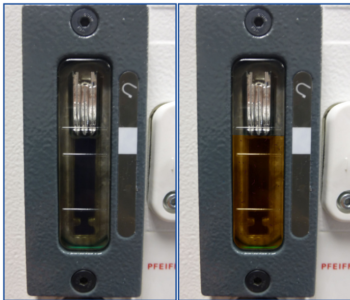
Figure 13: Pfeiffer Alcatel Adixen 2015SD rotary vane pump (P102310) with clean oil (left) and mildly dirty oil (right). On most rotary vane pumps, the oil condition can be determined by viewing it through a watch glass. As the oil degrades, its color darkens from clear, to yellow, to brown, to black. Its clarity decreases and its viscosity increases. Solid particles may be present. If other liquids mix with the oil an opaque emulsion may form with a matte appearance.
