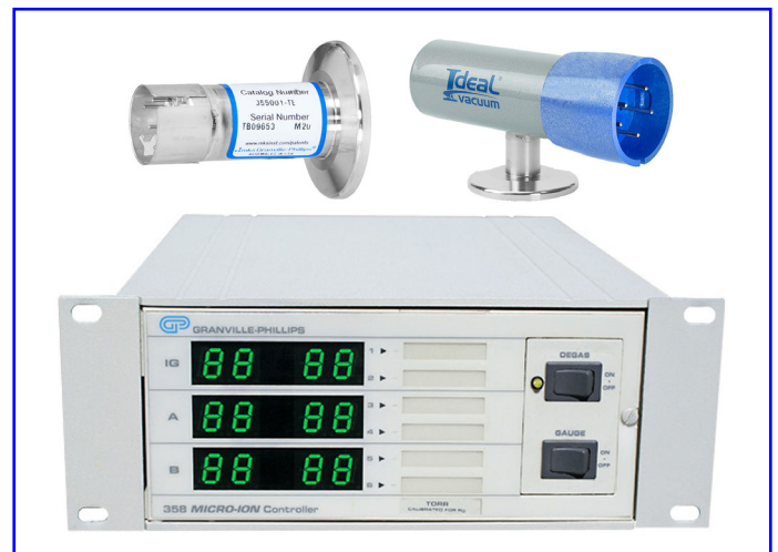
Figure 12: From left to right: MKS 355 hot cathode Micro-Ion® gauge (P1011205), IVP XGC-321 Convection-Enhanced Pirani Gauge (P1010260); bottom: MKS Granville-Phillips 358 hot cathode ion and convection-enhanced Pirani gauge controller (P1011910). The gauge controller automatically energizes the hot cathode ion gauge once the pressure measured by the convection-enhanced Pirani gauge drops below a set point.
