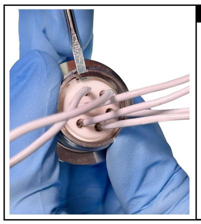
Place the screwdriver at the insert notch.
