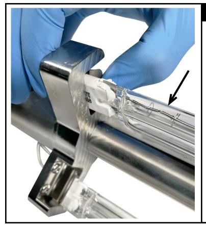
The lamp filament must be facing out from the center of the pendant.
