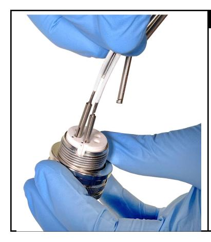
Take the two pins that were just crimped and insert them into the connector.
