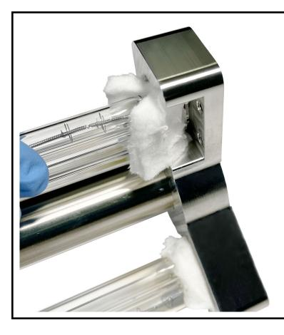
Slide the pendant into the bottom triple mount.
