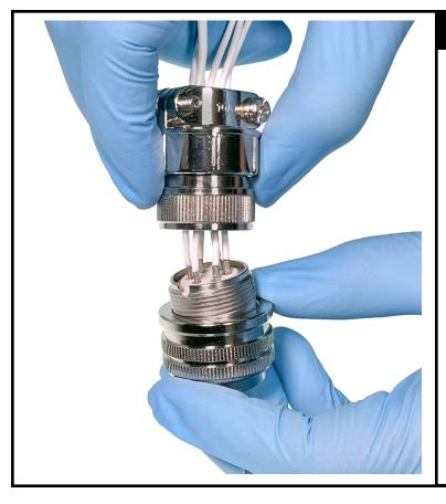
Screw the connector back together.
