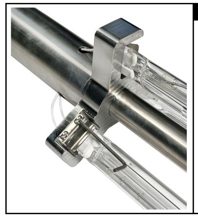
Screw down the retaining clip on the other end of the lamp (center of the pendant).
