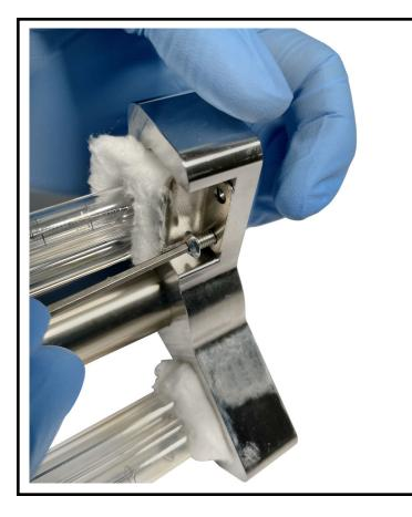
At the bottom of the pendant, remove the two retaining clip screws.
