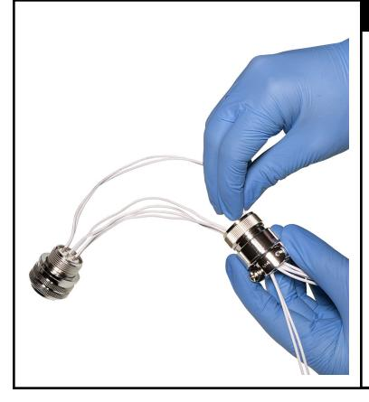
Pull the old lamp's two cut wires completely through the back of the connector.
