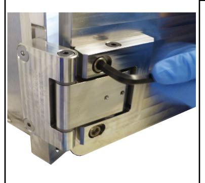
Use a 5/16" hex wrench to loosen the upper screw of the bottom hinge 1 full turn.
