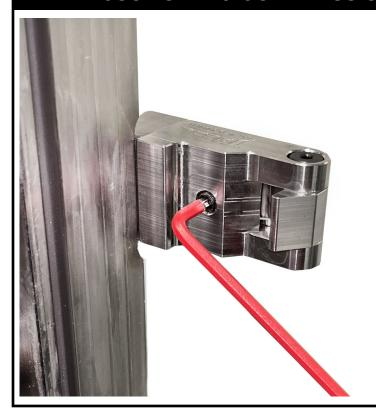
Adjustment of the O-ring compression may occasionally be necessary to ensure a good vacuum seal around the chamber door. Deformation or damage to the O-ring could cause a leak which, if not addressed, will result in poor vacuum performance.
