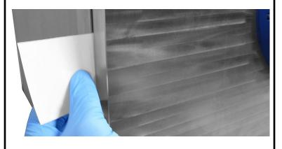
Insert a small piece of paper between the door and O-ring seal and slide it all around the chamber behind the door.
