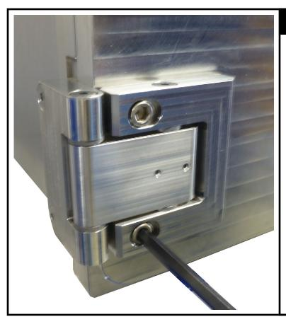
While holding the door in position, tighten the bottom hinge lower screw (only).
