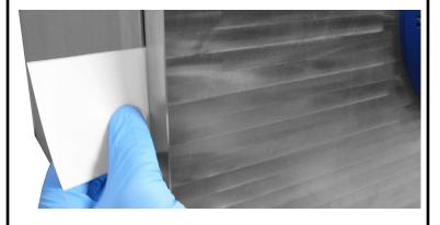
Insert a small piece of paper in between the door and O-ring seal and slide it all around the chamber behind the door.
