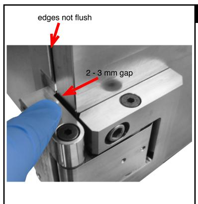
There should be a small gap (approximately 2 - 3mm) between the side of the bottom hinge and the side of the door when the latch is close to the catch.
