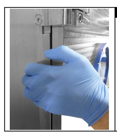
With the door latched, grasp and squeeze the door and chamber door frame tightly together below the top hinge.
