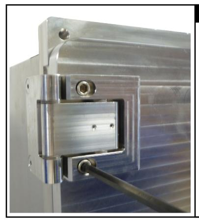
Use a 5/16" hex wrench to loosen the lower screw of the top hinge 1 full turn.
