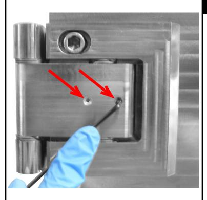
Use a 3/32" hex wrench to unscrew the four small set screws on the hinge faces (2 on each hinge).
