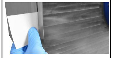
Insert a small piece of paper in between the door and O-ring seal and slide it all around the chamber behind the door.
