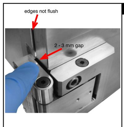
There should be a small gap (approximately 2 - 3mm) between the side of the bottom hinge and the side of the door when the latch is close to the catch.
