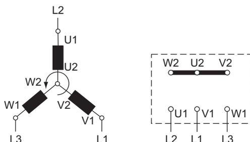
**Fig. 8: Star circuit for high voltage**
