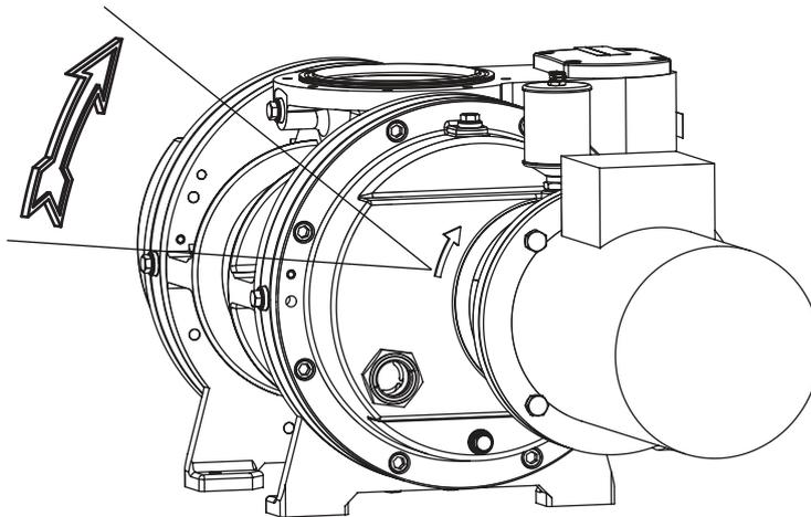
**Fig. 9: Check of direction of rotation**
