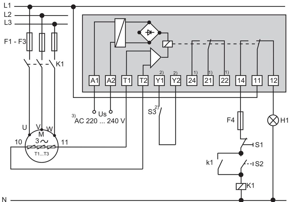
**Fig. 10: Connection example with PTC thermistor tripping unit**
