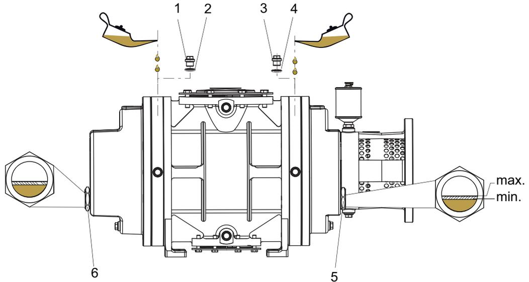
**Fig. 5: Filling with lubricant**
