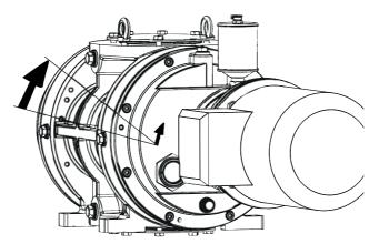
Fig. 7: Checking the direction of rotation
