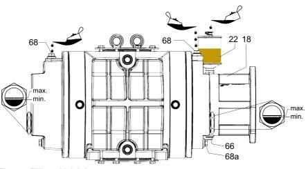
Fig. 4: Filling with lubricant
