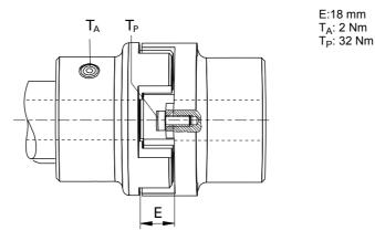
Fig. 13: Assembling the crown gear coupling at pump with standard coupling
