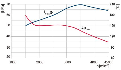
Fig. 15: Operating limits for differential pressure and discharge side gas temperatur
