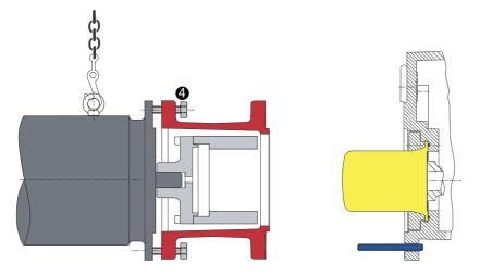
Fig. 14: Removing the motor – pump with magnetic coupling
