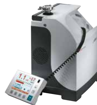
Detachable control panel (with approx. 2 m long cable)
