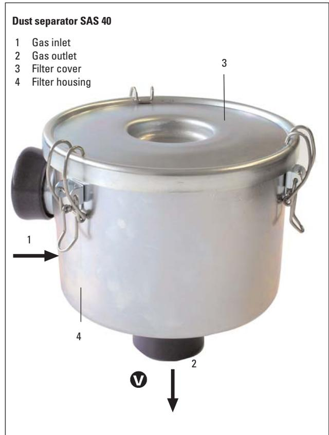
The SAS dust separators are installed in the intake line of vacuum pumps to prevent large dust particles from entering the pump. This increases the service life of the pump and the operating fluid.
