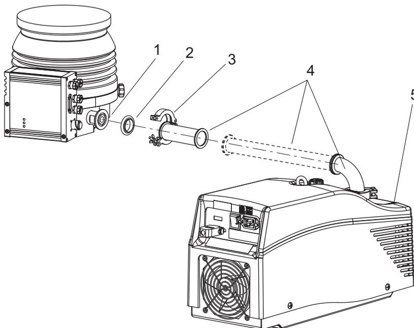
**Fig. 15: Example of fore-vacuum connection on HiPace 700**
