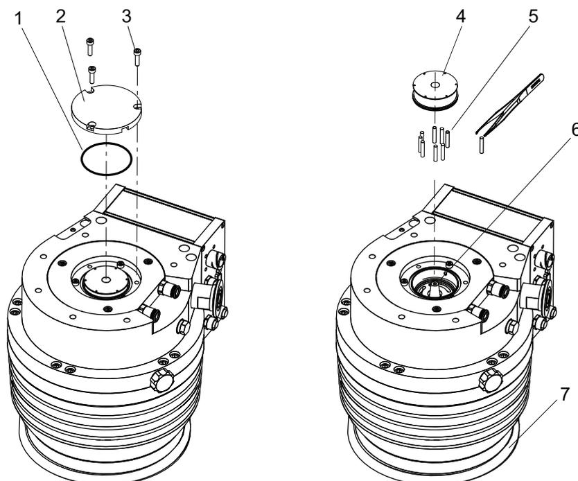
**Fig. 19: Removing the operating fluid reservoir**
