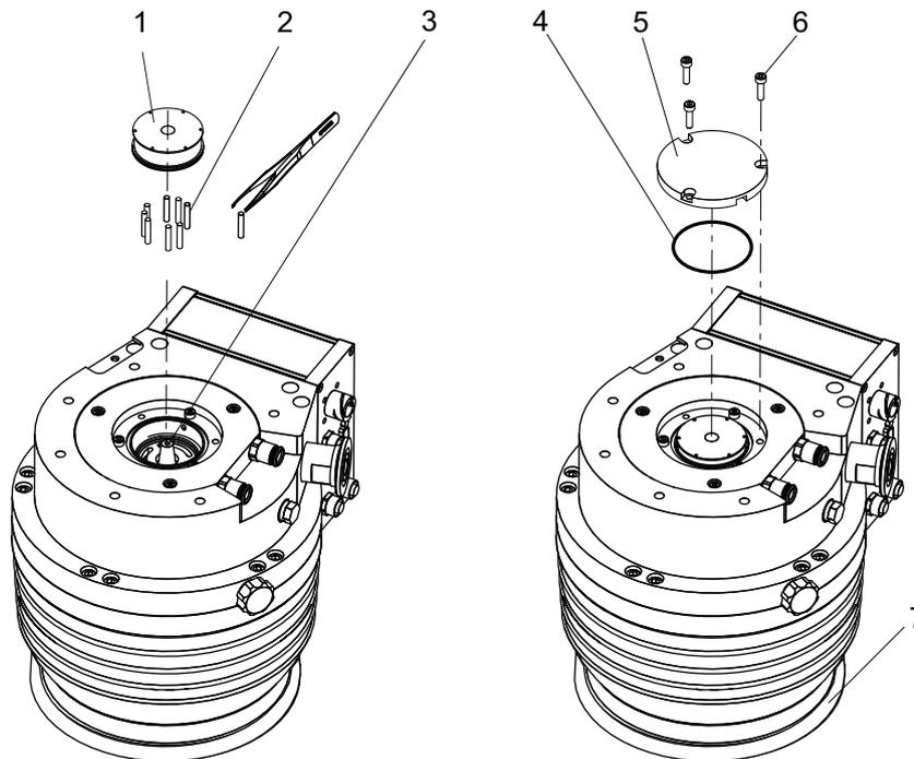
**Fig. 20: Installing the operating fluid reservoir**
