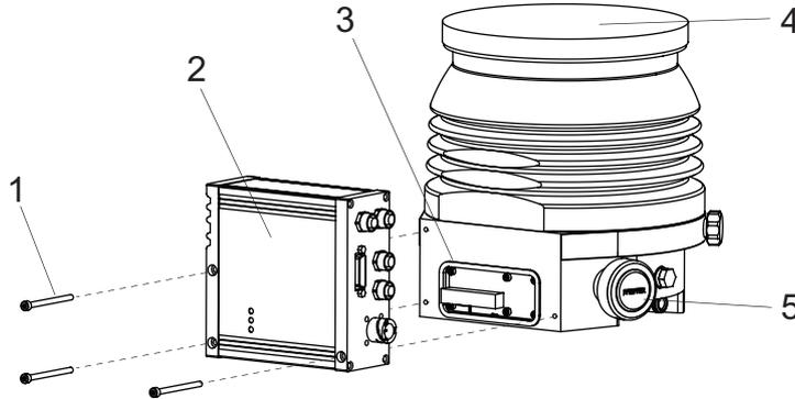
**Fig. 22: Installation of electronic drive unit TC 400**
