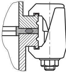
**Fig. 5: Flange connection ISO-K to ISO-F, bracket screws**
