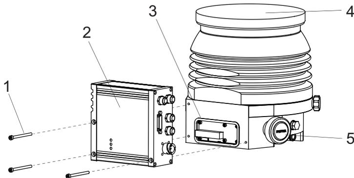
**Fig. 21: Removal of electronic drive unit TC 400**
