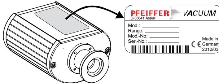
Fig. 1: Product identification on the rating plate
