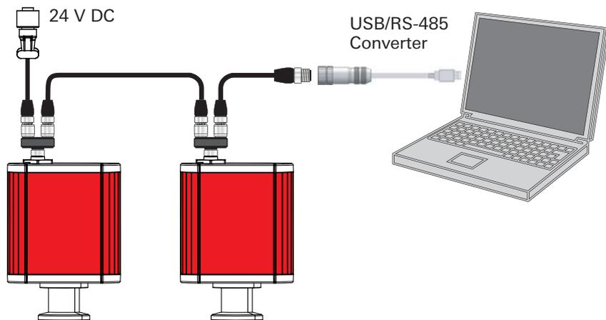
Fig. 5: Connections diagram gauge - USB/RS-485 converter
