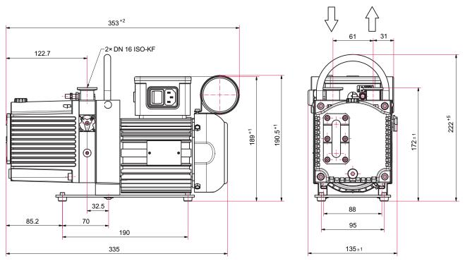
Fig. 19: Dimensions Duo 1.6, single-phase motor, 115/230 V, 50/60 Hz
