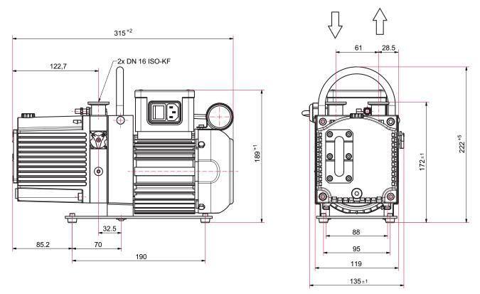
Fig. 20: Dimensions Duo 1.6, single-phase motor, 230-240 V, 50/60 Hz
