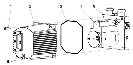
Fig. 14: Remove/fit rotary vane vacuum pump cap
