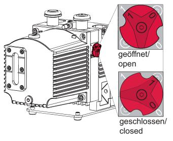
Fig. 11: Gas ballast valve
