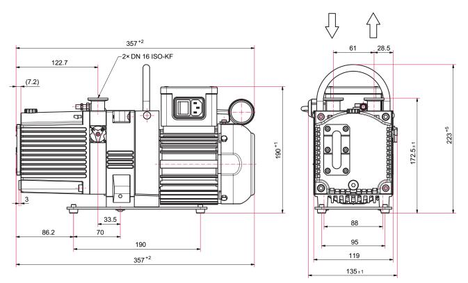
Fig. 23: Dimensions Duo 1.6 M, single-phase motor, 230-240 V, 50/60 Hz
