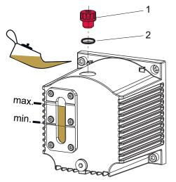
Fig. 10: Filling the operating fluid
