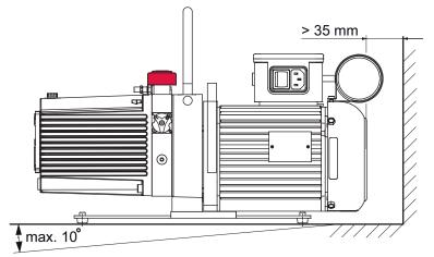
Fig. 5: Minimum distances and permissible inclination
