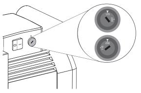
Fig. 9: Voltage selector switch on the terminal box
