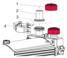
Fig. 6: Vacuum connection with flange connection
