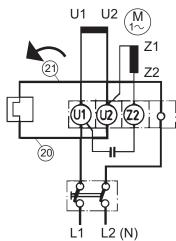
Fig. 8: Motor circuit diagram, single-phase motor with switch
