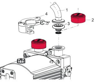
Fig. 7: Exhaust connection with flange connection
