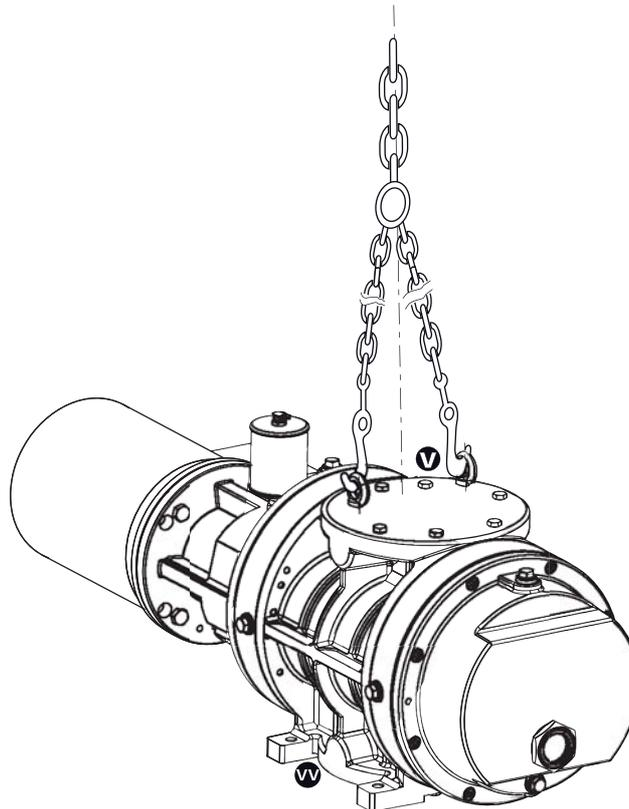
Fig. 3: Transporting the pump
