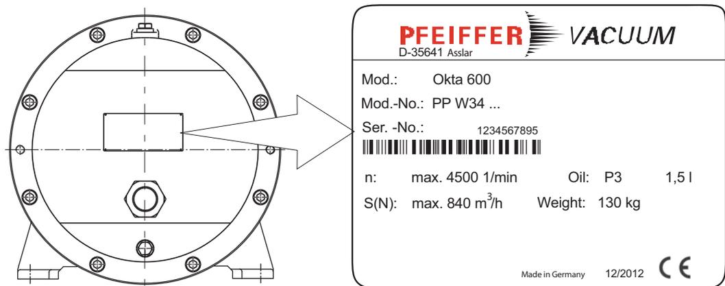
Fig. 1: Product identification on the rating plate (example)
