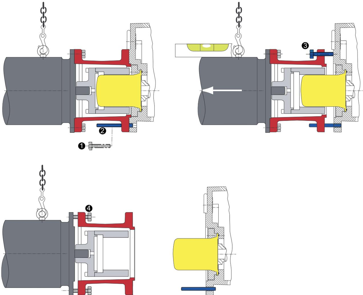
Fig. 14: Removing the motor – pump with magnetic coupling
