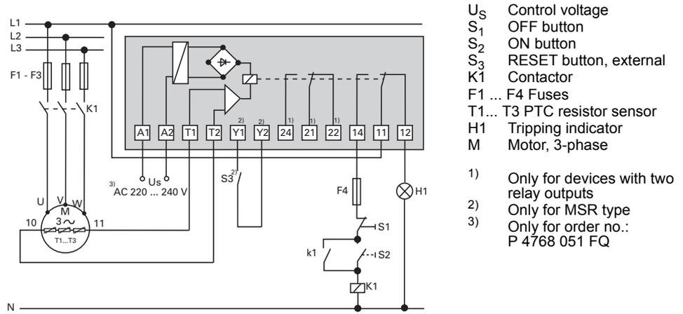
Fig. 8: Connection example for a three-phase AC motor with PTC resistor tripping device
