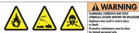
The user must label visibly the product to warn against pumped process gas that could be dangerous and toxic and could cause severe injuries or death. It precises that any preventive maintenance operation can only be performed by trained personnel.
