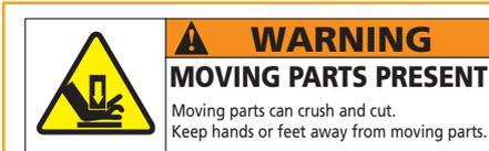
This label informs the user that moving parts present inside the pump could cause personal injury, like crushing or cutting. The user must keep all body parts away from moving parts.
