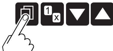
Fig. 27: Change from measuring mode to parameter mode
