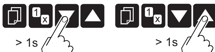
Fig. 24: Switching gauges on and off
