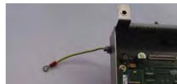
Introduce horizontally the support plate (1), with wiring harnesses first: check that wiring harnesses come out (2).
