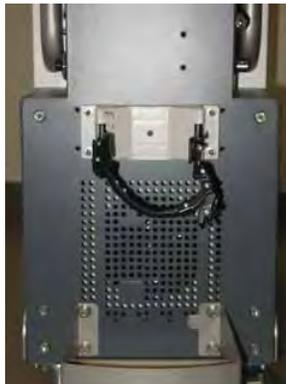
Bottle holder fixed on the leak detector
