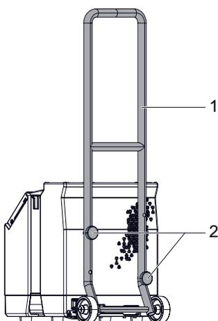
1 Cart      2 Fixing screws delivered with the cart
