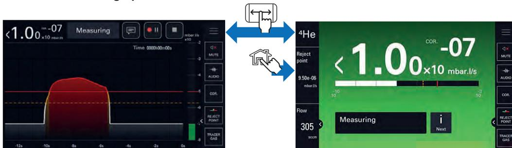
Access to the graph screen, menus and locked function keys
