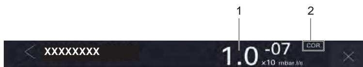
1 Digital display of leak rate and its unit
