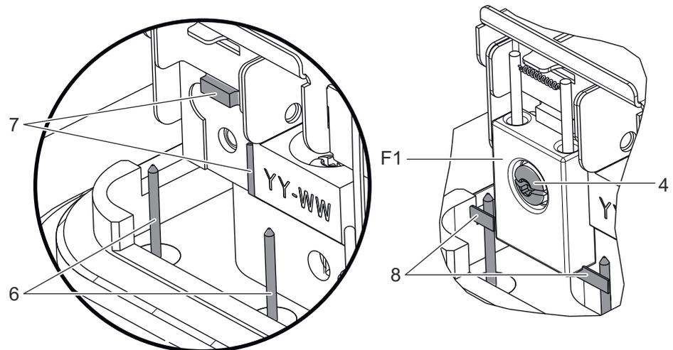
Fig. 4: Positioning the filament
