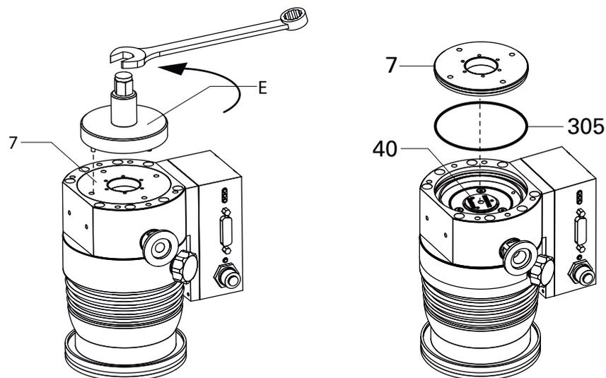
**Fig. 6: Assembly / Disassembly of the operating fluid reservoir**
