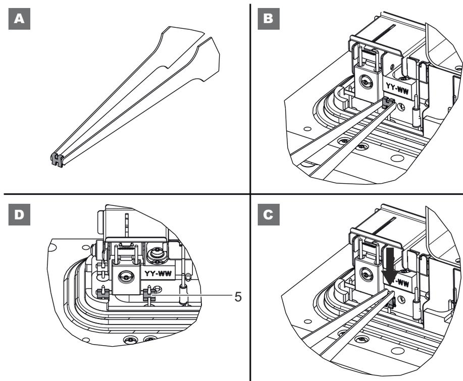
Fig. 5: Fitting of the fastening clip
