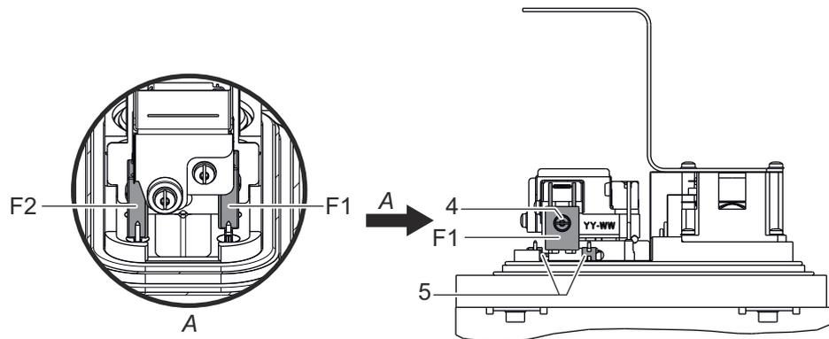
Fig. 3: Dismantling the filament
