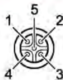
Fig. 12: "RS-485" connection (5-pole Binder M12 socket)
