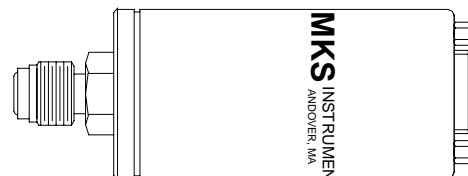
Figure 5: Acceptable Horizontal Mounting Positions
