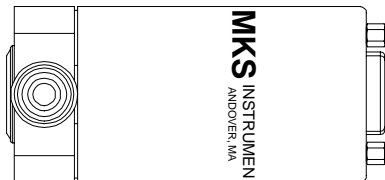
Figure 5: Acceptable Horizontal Mounting Positions
