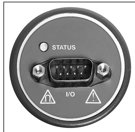
Figure 5: Status LED and Electrical Connector
