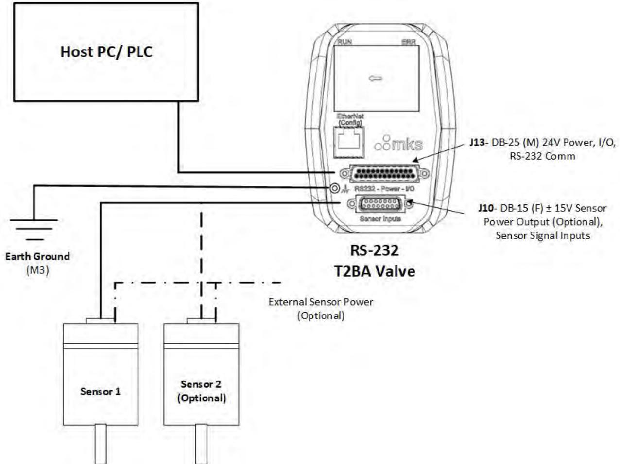
Figure 7: Typical System Configuration
