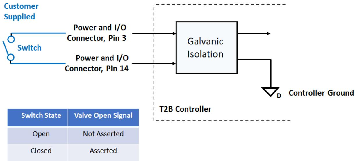
**Figure 8: Example of Valve Open Override Connection (Input)**
