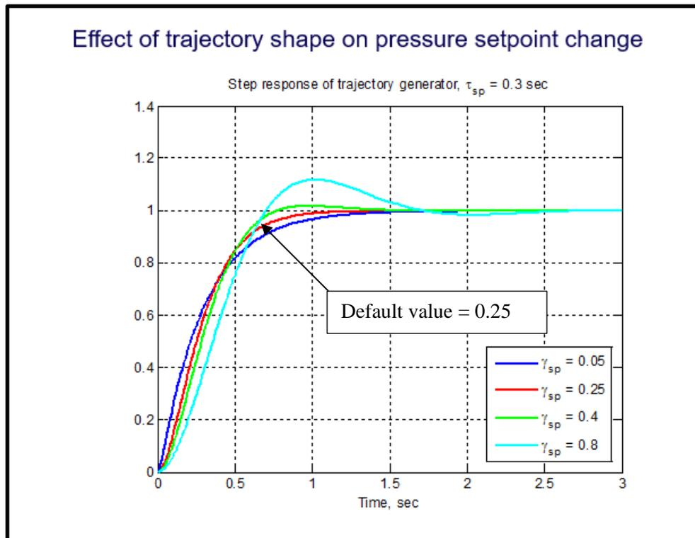
Figure 17: Pressure Setpoint Trajectory Shape Sensitivity Example
