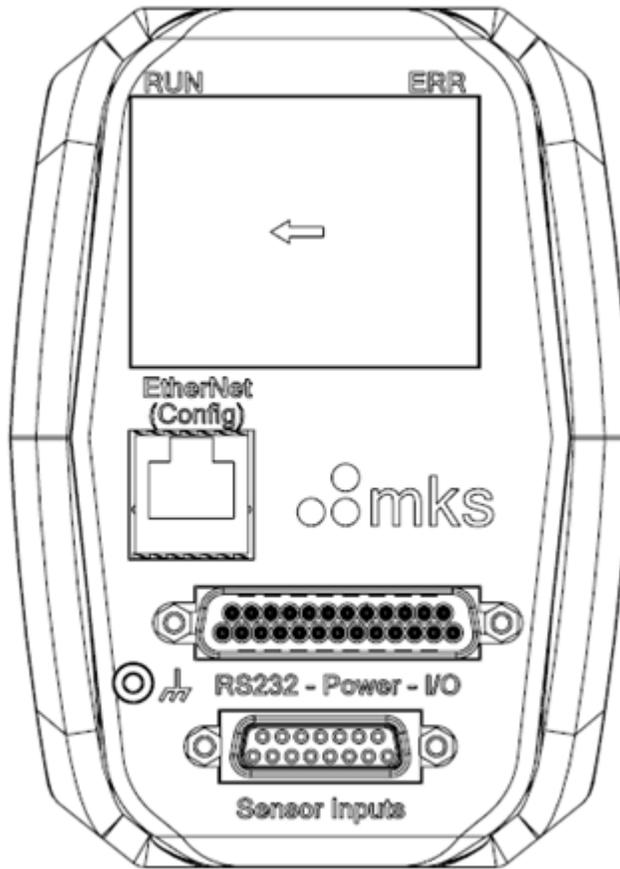
Figure 4: Top View of the T2BA Butterfly Valve (LCD Version of RS-232 I/O Interface)
