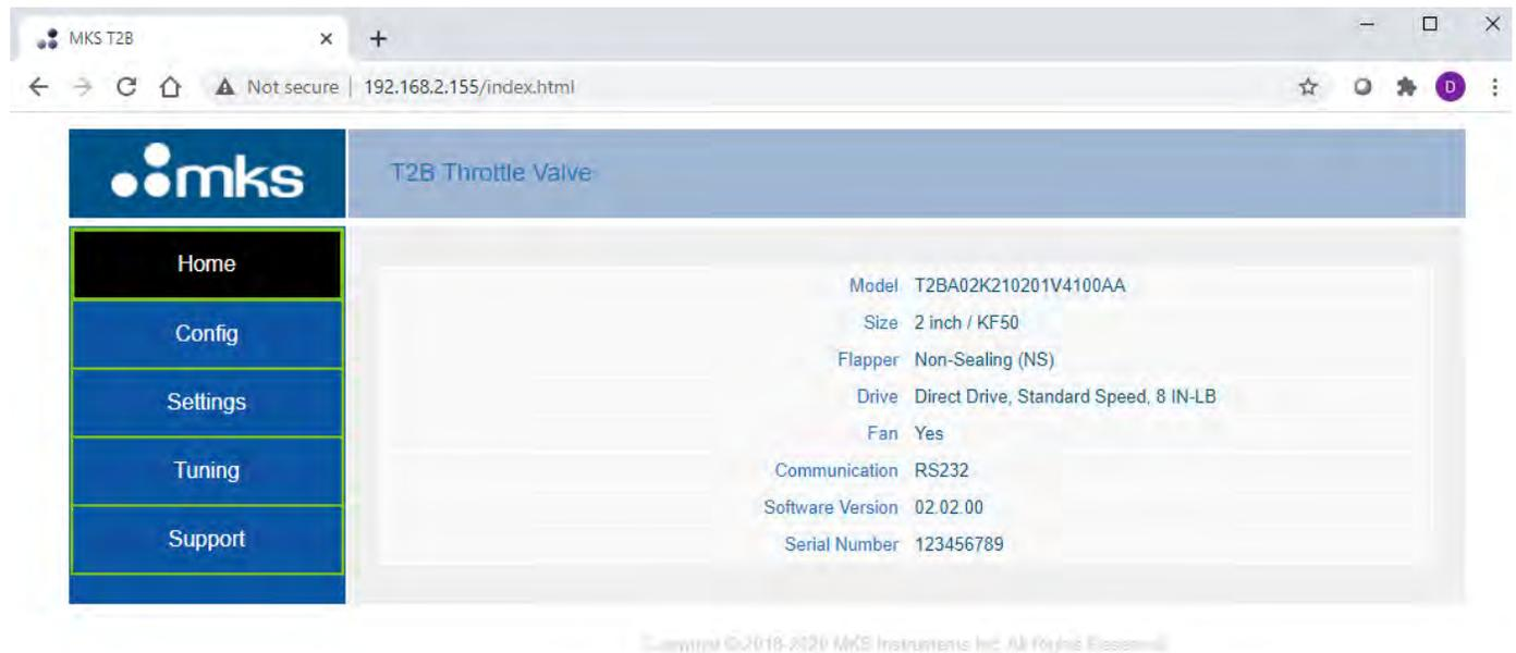
Figure 24: T2BA Butterfly Valve Embedded Interface (Home Page)
