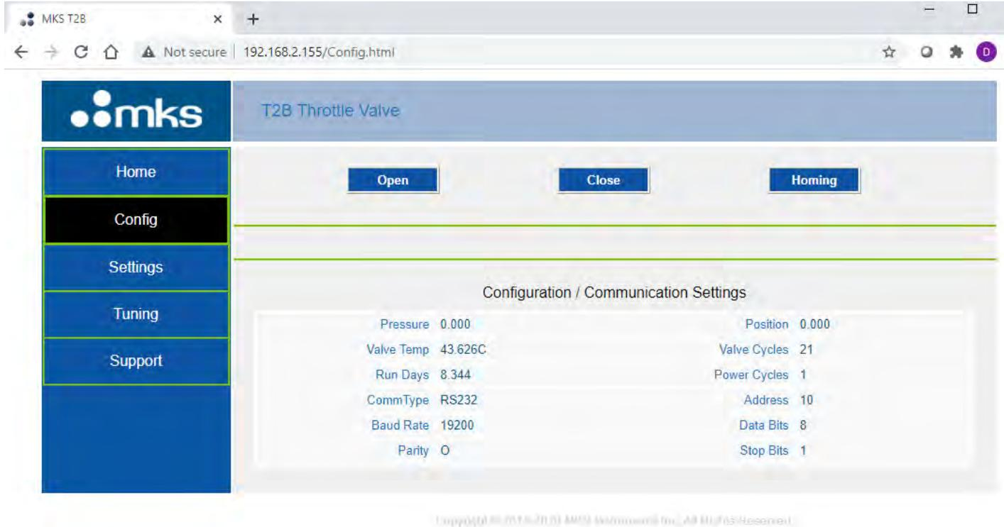
Figure 25: T2BA Butterfly Valve Embedded Interface (Configuration Page)
