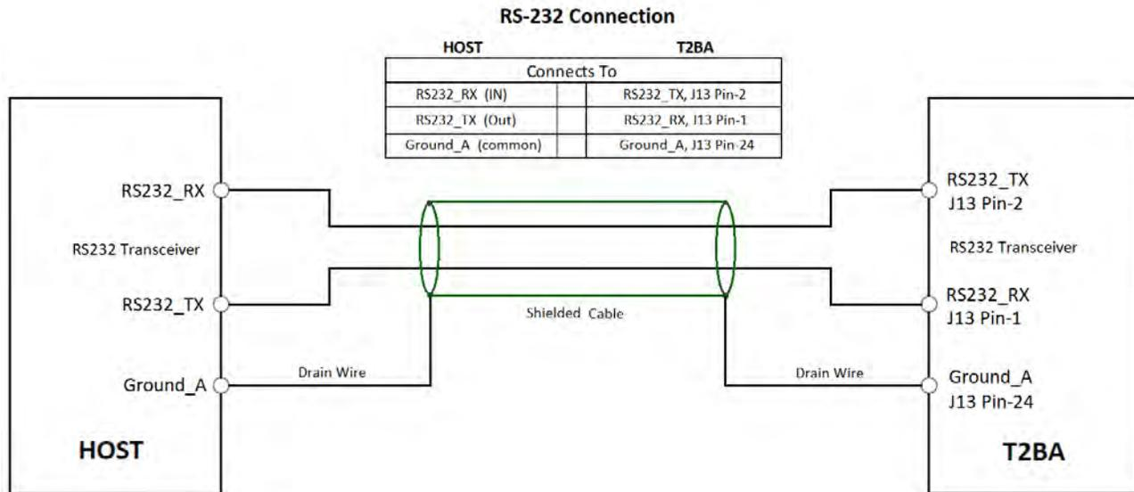
**Figure 9: T2BA RS-232 Electrical Connection to Network**
