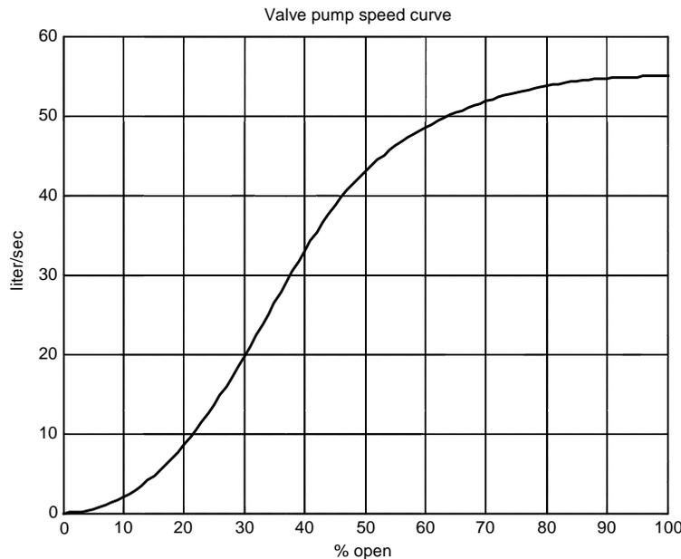
**Figure 14: Typical Chamber Pump Speed Curve**
