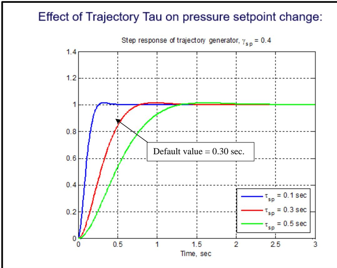
**Figure 16: Pressure Setpoint Trajectory Tau Sensitivity Example**
