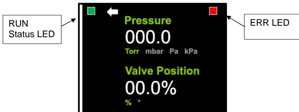
**Figure 11: T2BA Pressure / Position / Status Screen**
