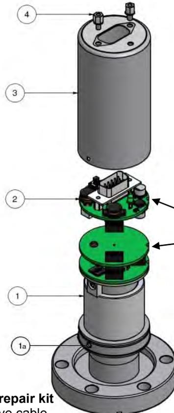
Printed circuit board alignment identification
