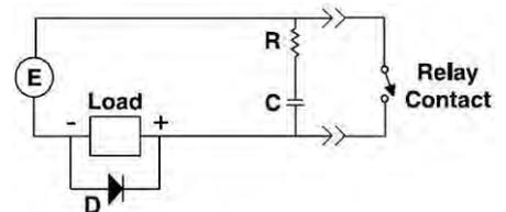
Note that  $R_{min} = 0.5 \Omega$  and  $C_{min} = 1 \times 10^{-9} \text{ F}$ . D is a fast transient suppression diode.
