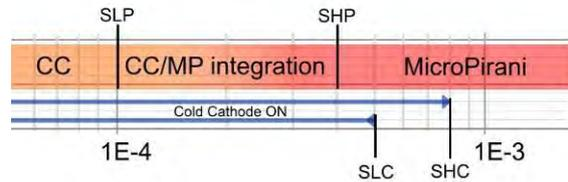
In some application it is preferred not to have the Cold Cathode (high voltage) turned on during vacuum process or during mass spectrometer analyzing. The 974B Cold cathode turn on pressure (SLC) and turn off pressure (SHC) can be changed by the user. Furthermore the high and low integration levels between the Cold Cathode reading and MicroPirani reading can be changed by the user.
