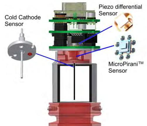
The cold cathode inverted magnetron utilizes a high voltage anode, cathode and a permanent magnet. Electrons are accelerated towards the anode and will ionize molecules by collision. The magnetic field deflects the electrons, causing them to spiral as they move across the magnetic field to the anode. This spiraling movement increases the opportunity for them to encounter and ionize the molecules. The ionization of the molecules creates an electric current as a function of the pressure.
