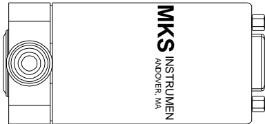
Figure 5: Acceptable Horizontal Mounting Positions
