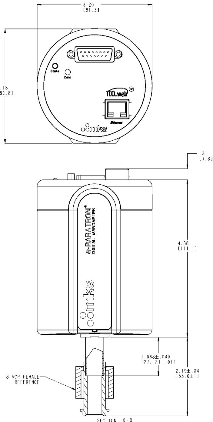
Figure 1: 62xE/E2xE Dimensions
