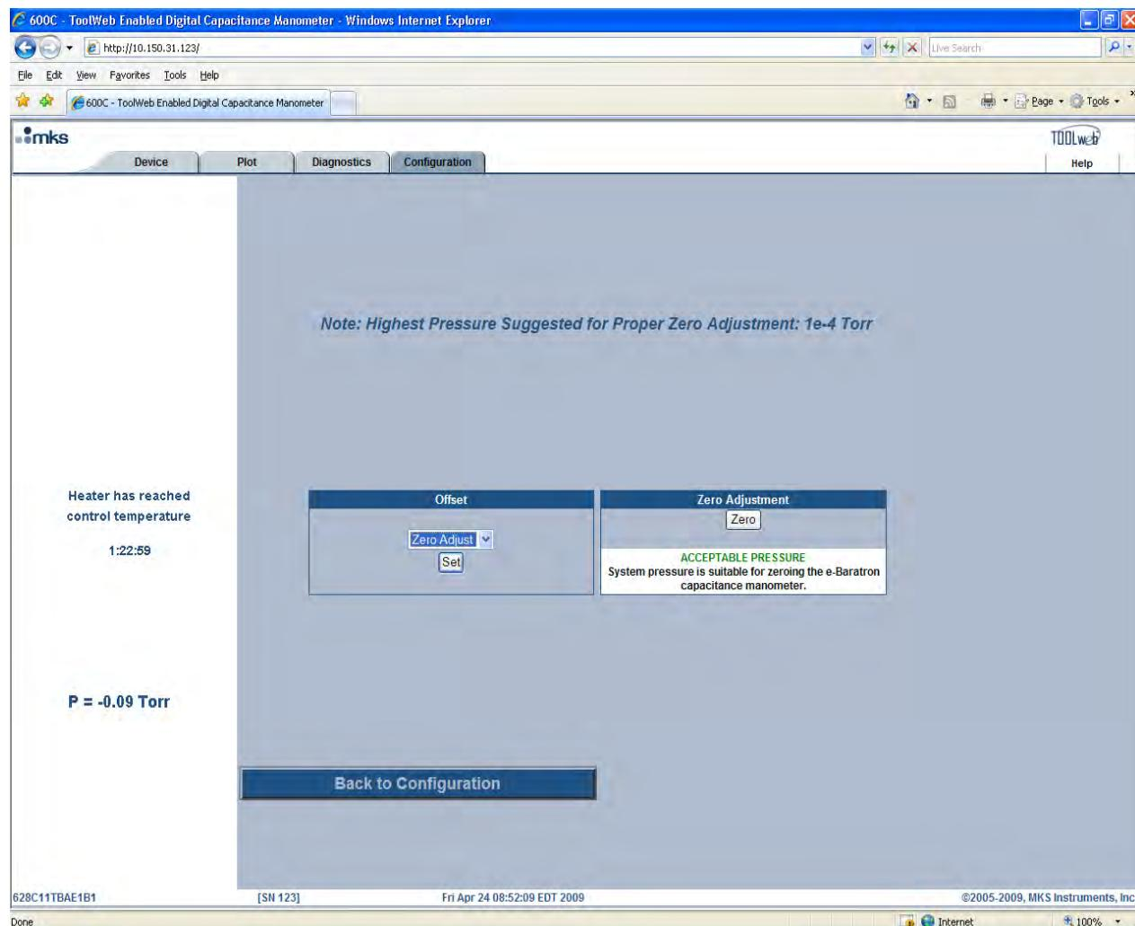
**Figure 13: Configuration/ Zero Adjustment with ‘Zero Adjust’ Option**
