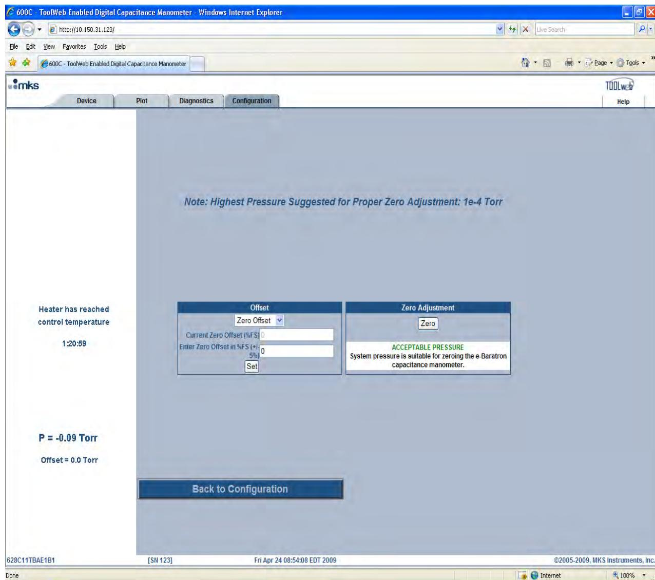
**Figure 14: Configuration/ Zero Adjustment with ‘Zero Offset’ Option**
