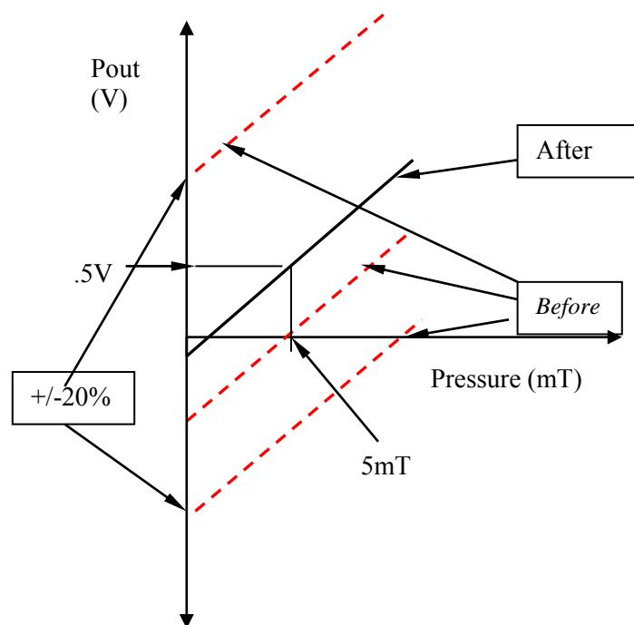
**Figure 18: Push-Button Zero with Zero Offset = x Fraction of FS**
