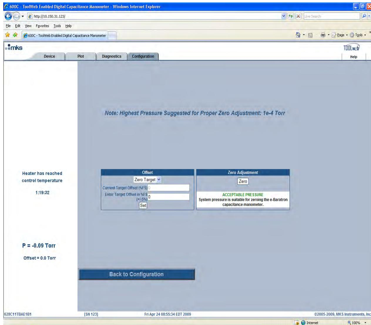
**Figure 15: Configuration/ Zero Adjustment with ‘Zero Target’ Option**
