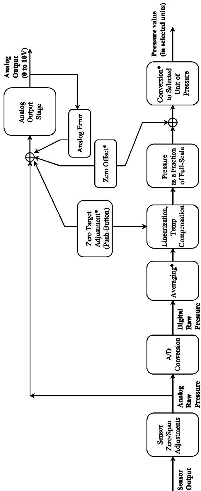
**Figure 4: Analog and Digital Pressure Calculation (Patented)**
