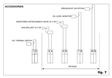
The electrical options installed on the pump are wired and have their respective connection terminals installed in the connection box.
