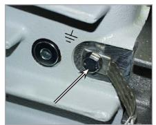
Fig. 3.7 Ground connection example
