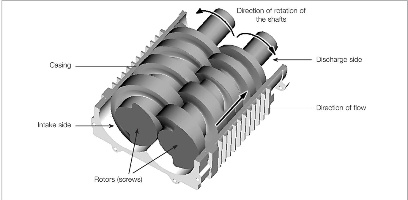
Fig. 1.1 Principle of operation of a screw pump
