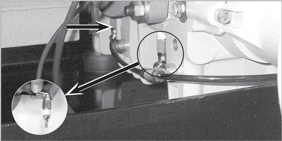
Fig. 5.4 Pull the hose lines off from the throttles
