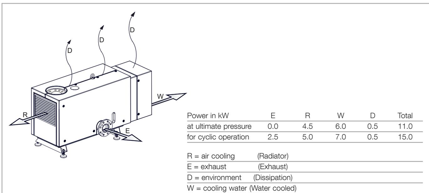
Fig.1.4 Heat dissipation at the SP 630 F
