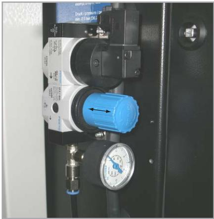
Fig. 5.7 Set up the pressure at the supply unit.
