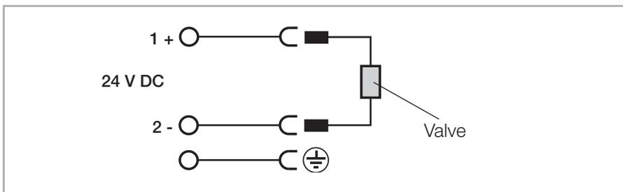
Fig. 3.13 Electrical connections at the purge gas valve
