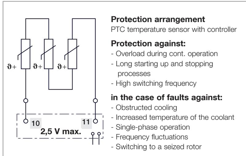
Fig. 3.2 Example for PTC temperature sensor circuit
