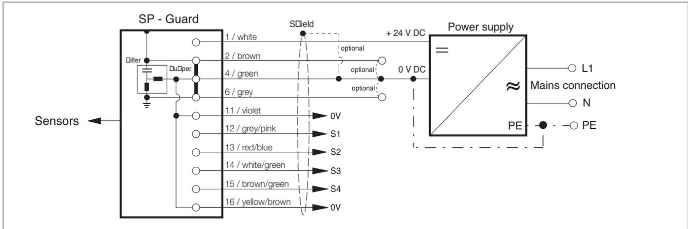
Abb. 3.7 Electrical connection - Power supply for status outputs
