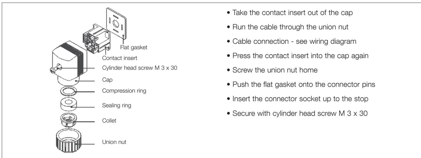
Fig. 3.11 Fitting the connector Bürkert 8376 for the gas ballast valve
