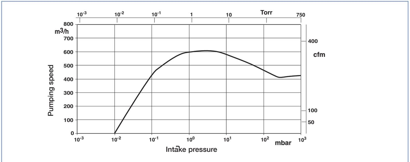
Fig. 1.5 Pumping speed curve for the SP 630/SP 630 F at 50 and 60 Hz
