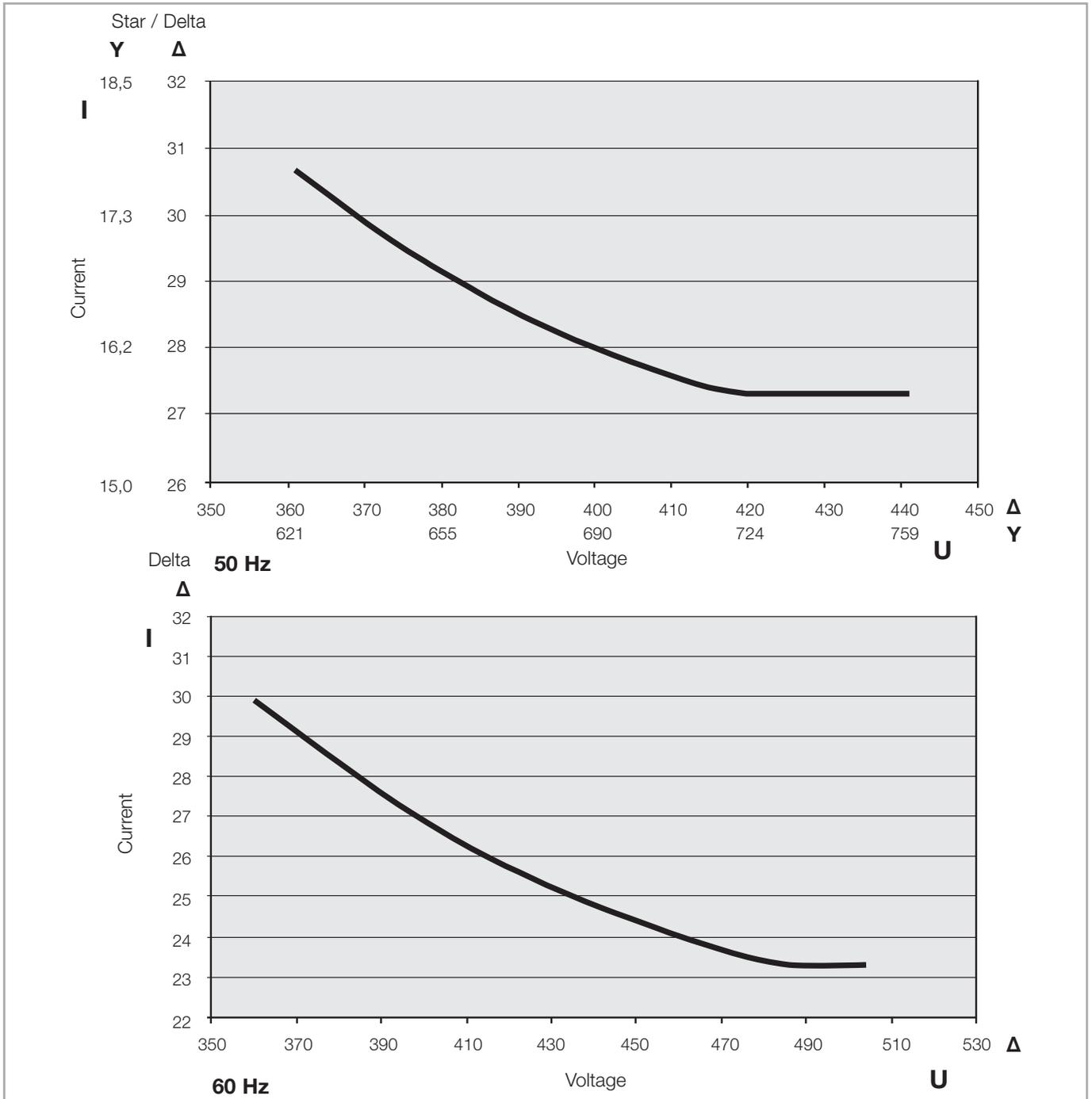
Diagram 1 Voltage/current diagram
