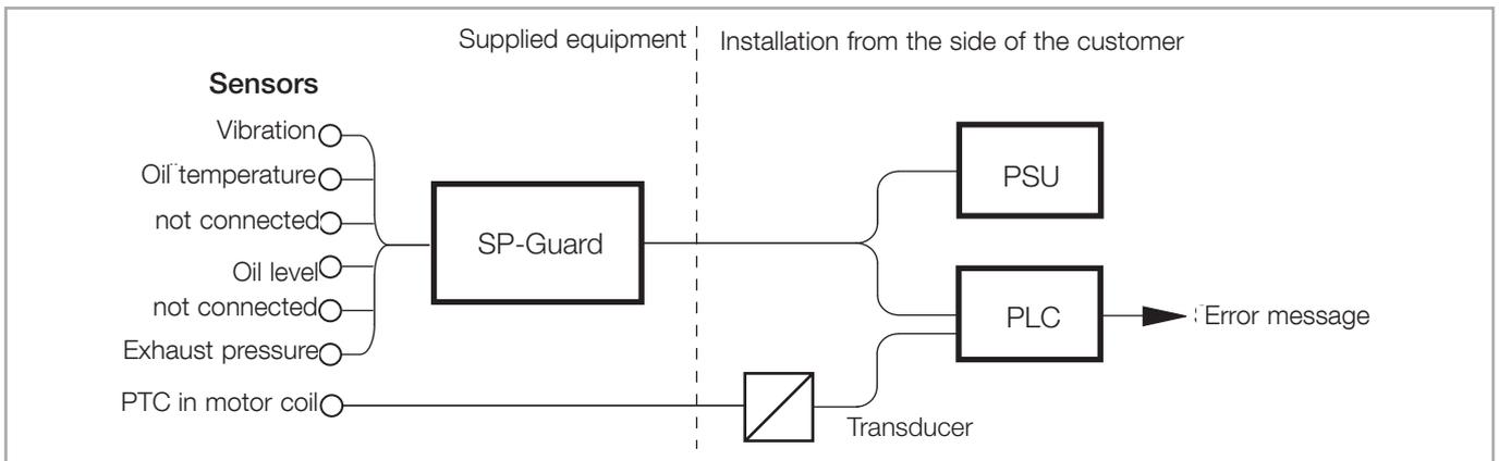
Fig. 1.8 Schematic depicting the operating principle of the monitoring system
