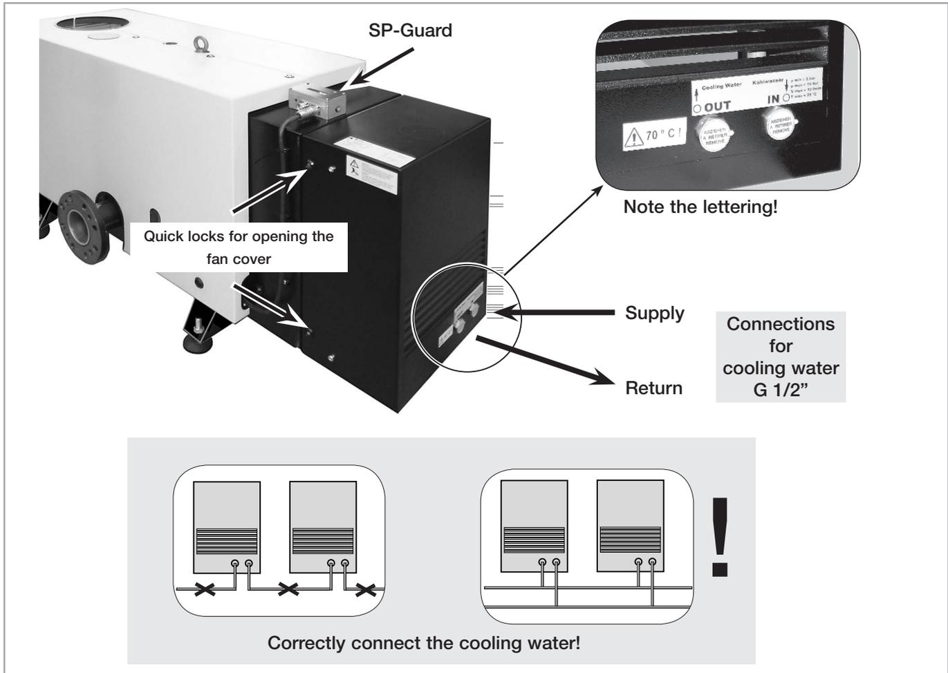
Fig. 3.4 SP 630 F - Connection of the cooling water
