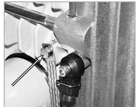
Fig. 3.6 Ground connection example
