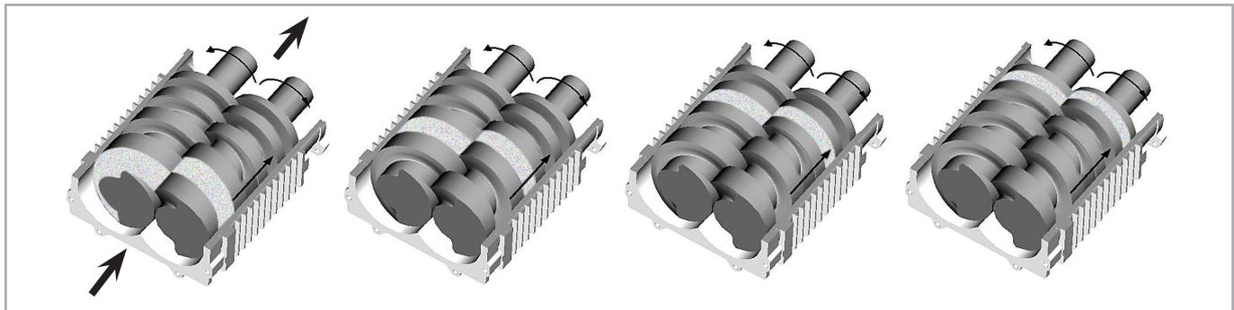
Fig. 1.2 Compression principle and the direction of pumping action within a screw pump
