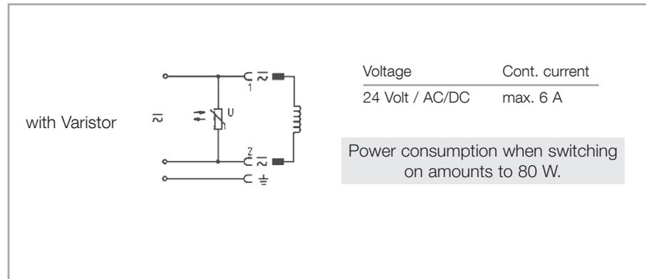
Fig. 3.10 Electrical connection at the solenoid valve
