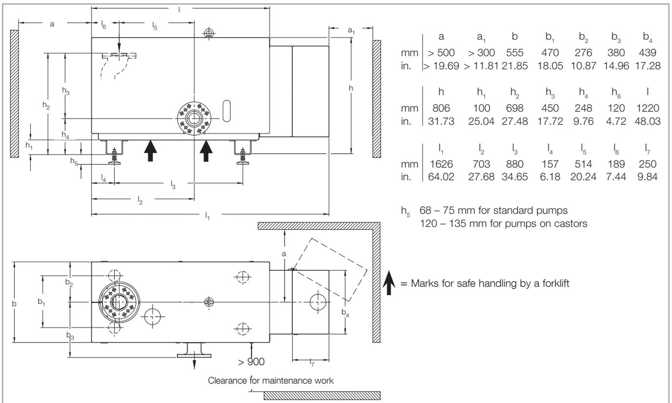
Fig. 1.6 Dimensional drawing for the SP 630
