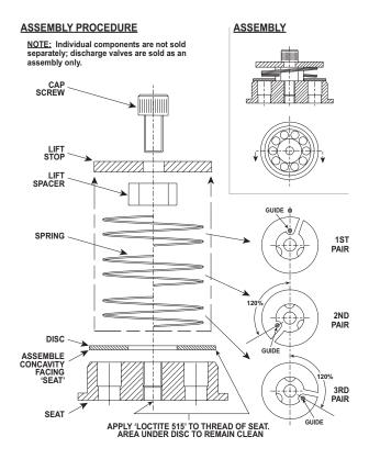
Figure 8-1 - Discharge Valve
