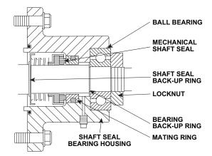
Figure 8-3 – KT-300, KT-500, KT-850 Shaft Seal and Bearing Housing
