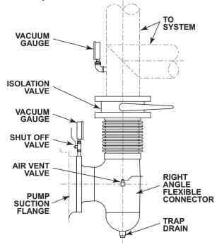
Figure 5-1 – Detailed Manifold Arrangement
