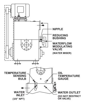
Figure 5-4 – Water Miser Installation
