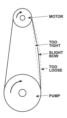
Figure 8-4 – V-Belt Tensioning
