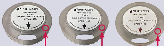
Font differences on the INFICON label can also be easily identified. The part number and frequency on an authentic INFICON cleanroom compatible carousel label is bold in font, as compared to the standard font for the description and lot code. In most of the counterfeit packaging seen to date, the part number and frequency has been printed in the same text as the description and lot code.
