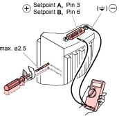
Using a screwdriver (max. ø2.5 mm), set the threshold of the selected switching function (Setpoint A, B) to the desired value UThreshold
