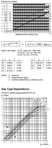
Calibration factors for the pressure range below 1 mbar
