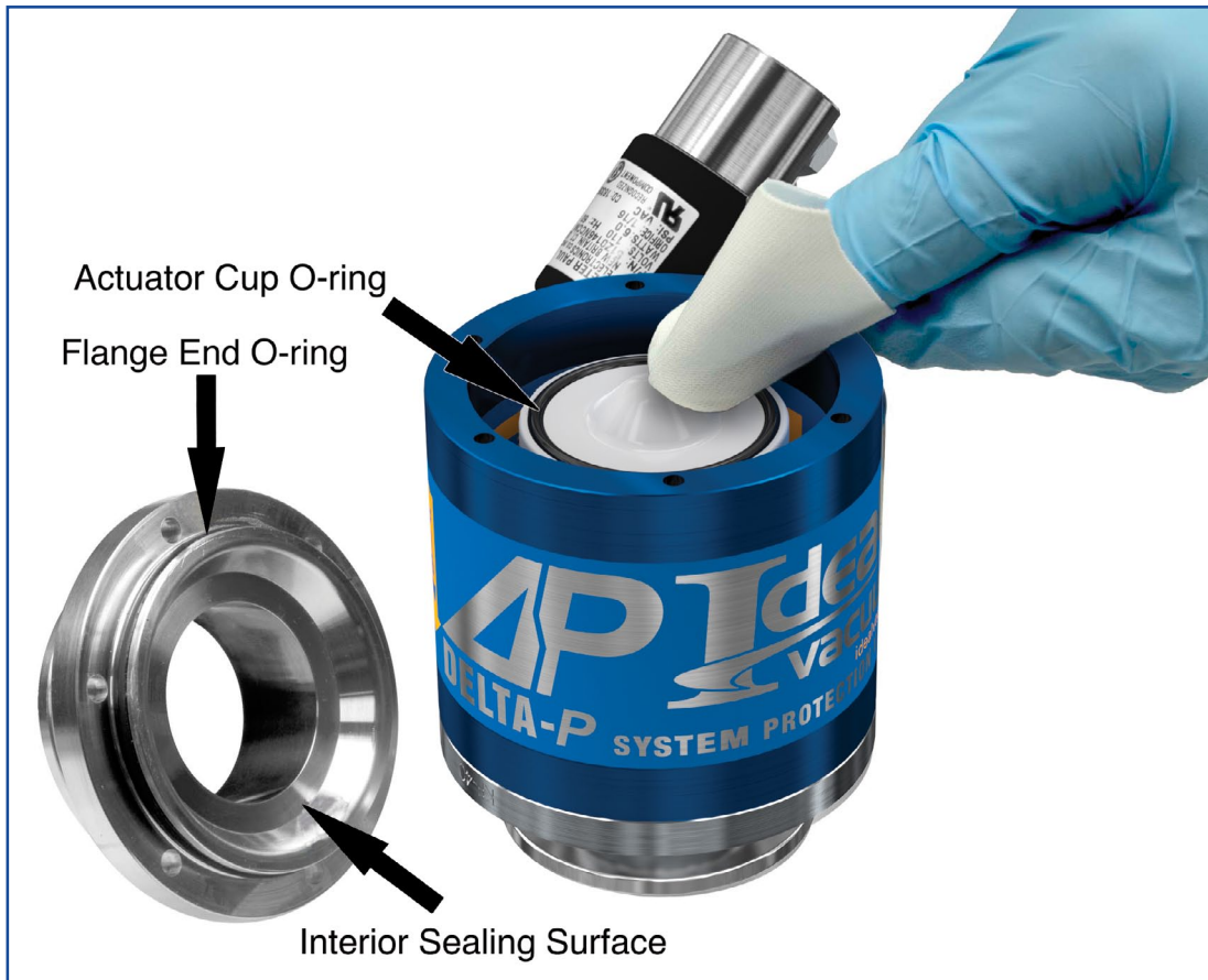
Figure 7 - Cleaning the Actuator Cup O-Ring
