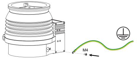
Fig. 17: Example: Connecting the grounding cable
