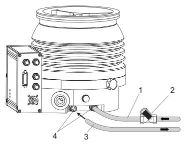
Fig. 16: Connecting the cooling water supply
