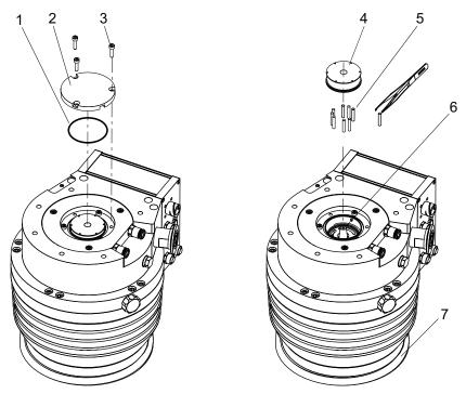
Fig. 19: Removing the operating fluid reservoir
