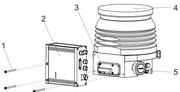
Fig. 22: Installation of electronic drive unit TC 400
