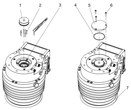
Fig. 20: Installing the operating fluid reservoir
