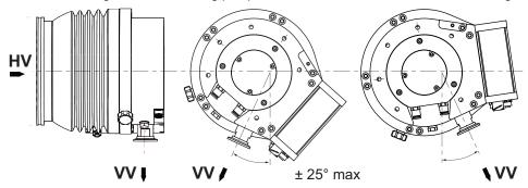
Fig. 4: Recommended alignment when using oil-sealed backing pumps
