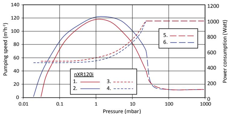
1. Pumping speed with gas ballast
