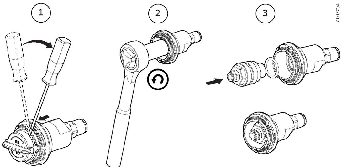
The manually operated gas ballast knob can be replaced by a gas ballast adaptor which enables external electrically actuated valves or a controlled gas supply to be used through a 1/4 inch push fit connector. To install the gas ballast adaptor:
