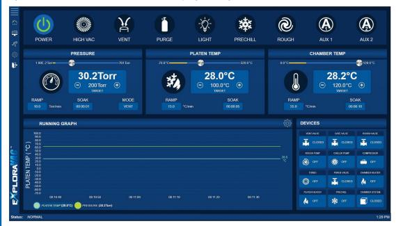
The Home Screen is the landing page for the software. It offers manual control of all components in the system and has three main sections: manual operation, running graph. and device panel. The manual operation section allows control over all installed devices. The running graph plots sensor output values as a function of time. The device panel reports the status of all devices and displays current operating parameters.
