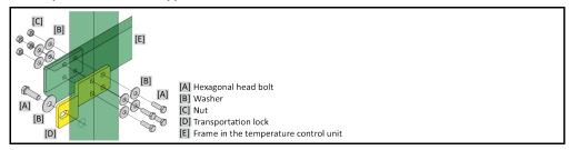
Remove the side panel on the temperature control unit to loosen and tighten the transportation locks.
