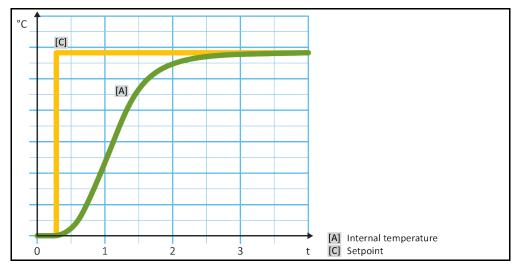
Internal, dynamic temperature control with possible overshooting of the temperature
