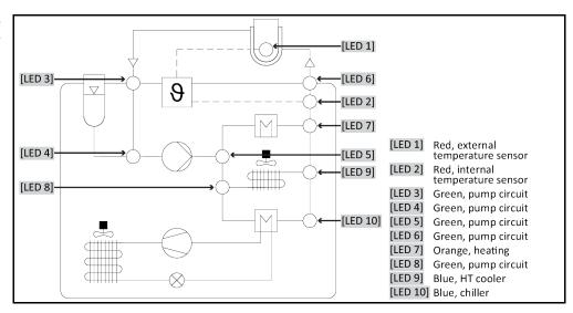
Components illustrated in the LED flow diagram
