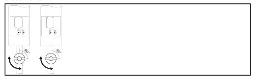
2.10.3.2.1 Closing the shut-off valves (locking the expansion vessel)
