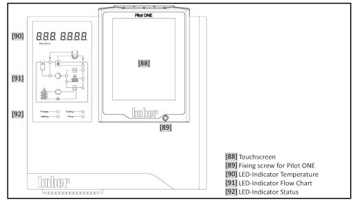
Description of the LEDs in the flow diagram
