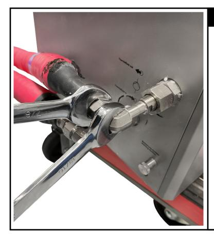
If the unit needs to be moved or transported, the platen and fluid hoses might have to be drained.
