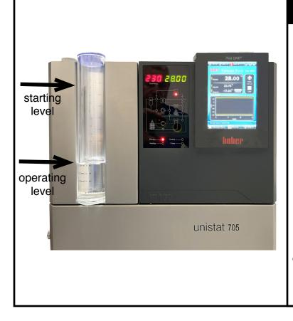
Allow the machine to circulate fluid for about 5 minutes. Then, press Stop.
